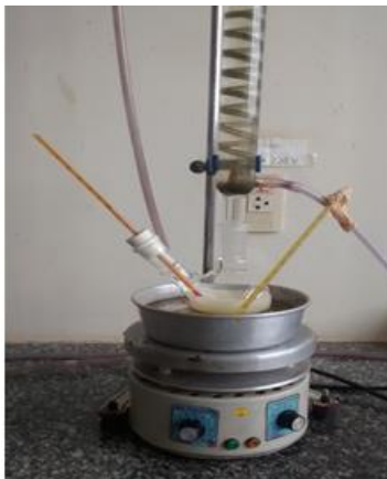
Figure 3 – Basic homogeneous transesterification process of gong oil
